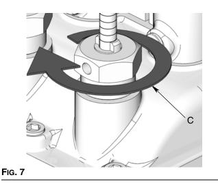
• Turn the feed adjustment nut (C) counter-clockwise to reduce the pump stroke and delivery (FIG. 8).
